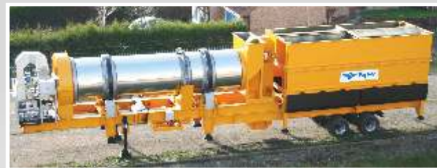
Mobile cold feed unit, dryer and burner
