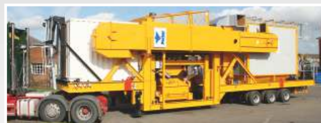
Mobile control cabin, mixing section including primary and secondary dust
